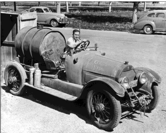
Early Fire Truck - Jack Hahn, a volunteer fireman, drives the 1918 Cadillac equipped as a Cotati fire truck. It had tanks for soda and acid, which, when mixed, produced pressure to pump water from the big drum.
